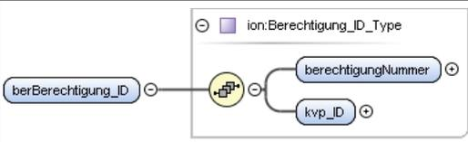
The diagram shows the structure of the <code>tns:Berechtigung_ID_Type</code> element. It is a complex type containing two child elements: <code>berechtigungNummer</code> and <code>kvp_ID</code> . Each child element is shown with a cardinality of 1 and a required status (indicated by a circle with a plus sign). |
