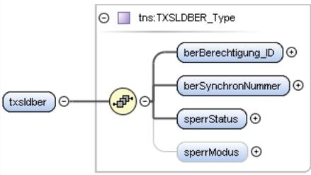
The diagram shows the structure of the <code>tns:TXSLDBER_Type</code> element. It is a complex type containing four child elements: <code>berBerechtigung_ID</code> , <code>berSynchronNummer</code> , <code>sperrStatus</code> , and <code>sperrModus</code> . Each child element is shown with a cardinality of 1 and a required status (indicated by a circle with a plus sign). |
