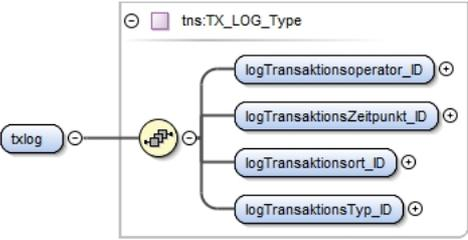
The diagram shows a tree structure for the tns:TX_LOG_Type element. The root node is 'txlog'. It has four child nodes: 'logTransaktionsoperator_ID', 'logTransaktionsZeitpunkt_ID', 'logTransaktionsort_ID', and 'logTransaktionsTyp_ID'. |
