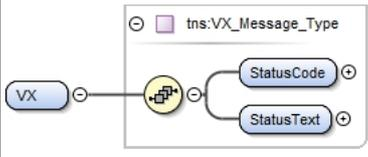
The diagram shows the structure of the tns:VX_Message_Type element. It is a root element (VX) containing a complex content type (represented by a yellow circle with a plus sign) which contains two child elements: StatusCode and StatusText.                                                                                                                       |
