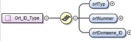
The diagram shows a complex type 'Ort_ID_Type' containing three elements: 'ortTyp', 'ortNummer', and 'ortDomaene_ID'. Each element is represented by a rounded rectangle with a small circle containing a plus sign, indicating they are optional. They are connected to the parent type by lines.                                                                                                                                     |
