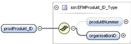
The diagram shows the structure of the tns:EFMProdukt_ID_Type element. It is a complex type containing two child elements: produktNummer and organisationID. Each child element is represented by a rounded rectangle with a plus sign and a circle, indicating a required one-to-one relationship. |
