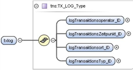
The diagram shows the structure of the tns:TX_LOG_Type element. It is a complex type containing four child elements: logTransaktionsoperator_ID, logTransaktionsZeitpunkt_ID, logTransaktionsort_ID, and logTransaktionsTyp_ID. Each child element is represented by a rounded rectangle with a plus sign and a circle, indicating a required one-to-one relationship. |
