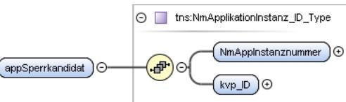
A UML class diagram fragment showing an element named "appSperrkandidat" with a multiplicity of 0..1. It has two directed associations: one to "NmAppInstanznummer" with multiplicity 0..1 and one to "kvp_ID" with multiplicity 1..1. Both "NmAppInstanznummer" and "kvp_ID" are shown as attributes of a base type "tns:NmApplikationInstanz_ID_Type". |          |         |           |       |
