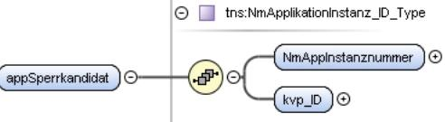
A UML class diagram fragment showing an element named "appSperrkandidat" with a multiplicity of 0..1. It has two directed associations: one to "NmAppInstanznummer" with multiplicity 0..1, and another to "kvp_ID" with multiplicity 1..1. Both "NmAppInstanznummer" and "kvp_ID" are shown as attributes of a class named "tns:NmApplikationInstanz_ID_Type". |          |         |           |       |
